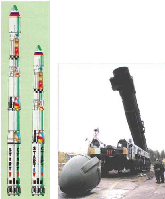
Fig. 5. The Russian 'Start' (left) and 'Start-1' launch vehicles and the 'Topol' missile from which they are derived.
