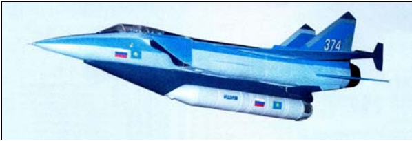
Fig. 2. A model of the 'Ishim' Kazakhstan launch system's MiG-31I carrier aircraft with the suspended launch vehicle.
