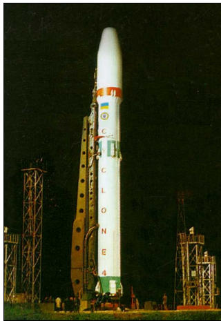
Fig. 4. The “Cyclone-4” Ukrainian/Brazilian launch vehicle would launch up to 1600 kg of payload into a GTO from its launch site in the near-equatorial Alcantara test range
