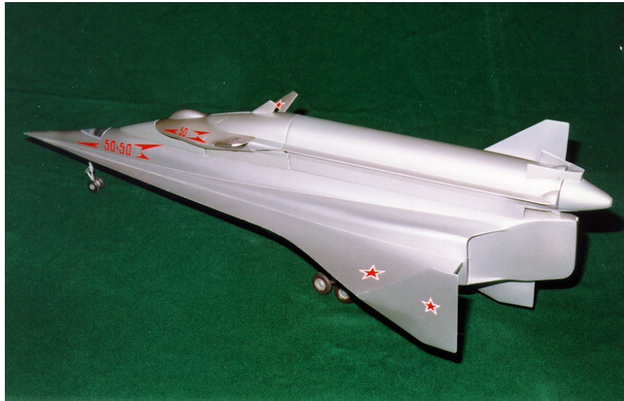
Fig.1. The 'Spiral' aerospace system in the take-off configuration
