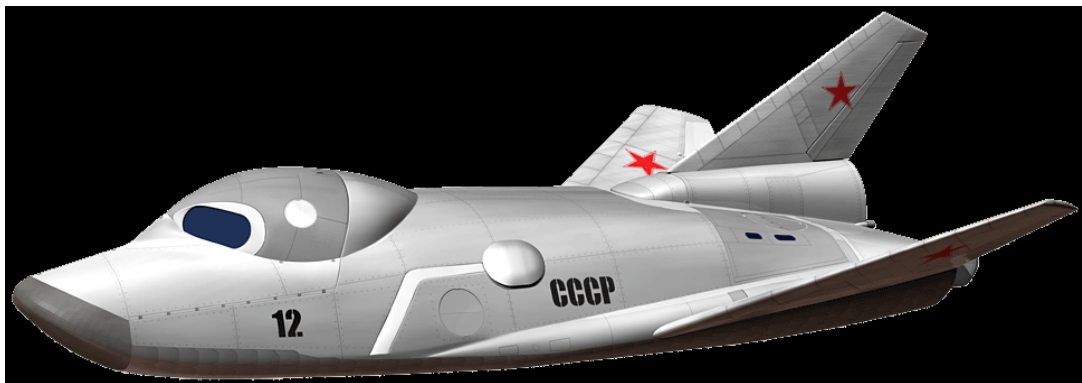
Fig.2. The 'Spiral' system's Orbital Plane (OS) in flight configuration
