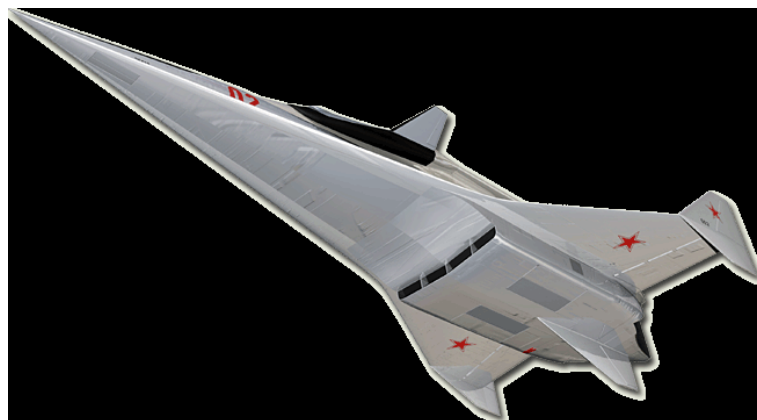
Fig.3. The 'Spiral' system's Hypersonic Airplane Booster (GSP) in flight configuration
