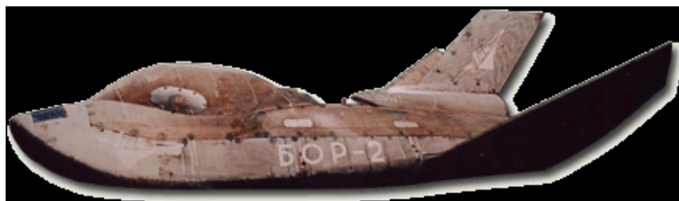
Fig.5. An external view of the BOR-2 sub-orbital experimental vehicle
