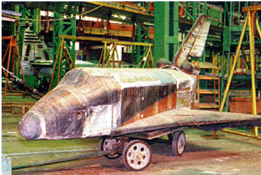
Fig.8. BOR-5 had the 'Buran' Orbiter's external configuration
